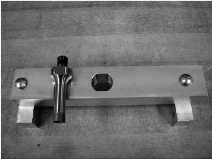
FIGURE 8 Position of tool holding for observation of tool lateral face.
