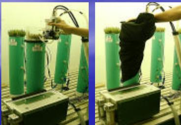
Figure 1. Licor 6400 (Li-6400) with a custom surface chamber was used to measure net photosynthesis (left) and total respiration rates (right). For respiration measurements, a black cloth covered the chamber which prevented light penetration and photosynthesis.
