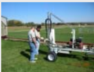
Figure 2. A hydraulic soil probe was used for collection of root cores in this study
