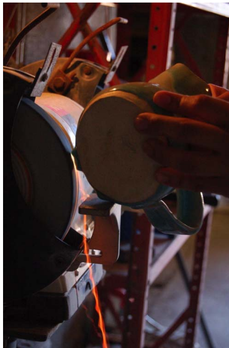
Ceramics one student, Maleri Malekyar, works on a machine called a grinder, used to clean up drips from firing, that are now considered to be glass.
