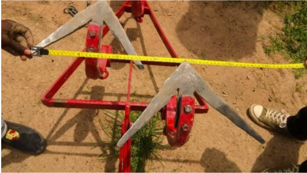
Low-crown, low pitch-angle sweeps built by the local blacksmith with locally available materials reduced implement draft by 21% and improved weed control.
