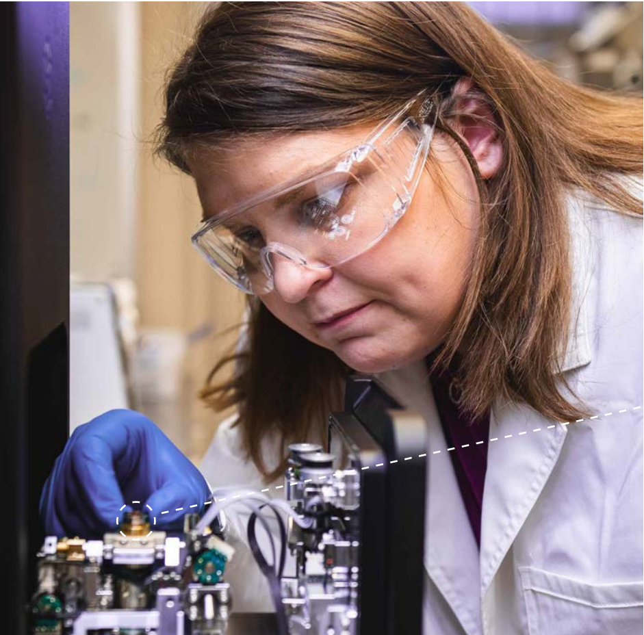
K-State nano-entomologist Amie Norton, left, places a stub containing a red flour beetle treated with micro eggshell particles, shown enlarged at right, into a scanning electron microscope in order to get an image of the particles that are present on the beetle.
