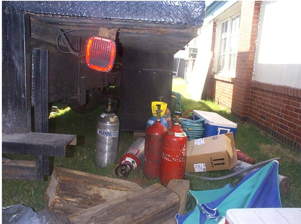
**Violation:** Improper storage of compressed gas cylinders.
