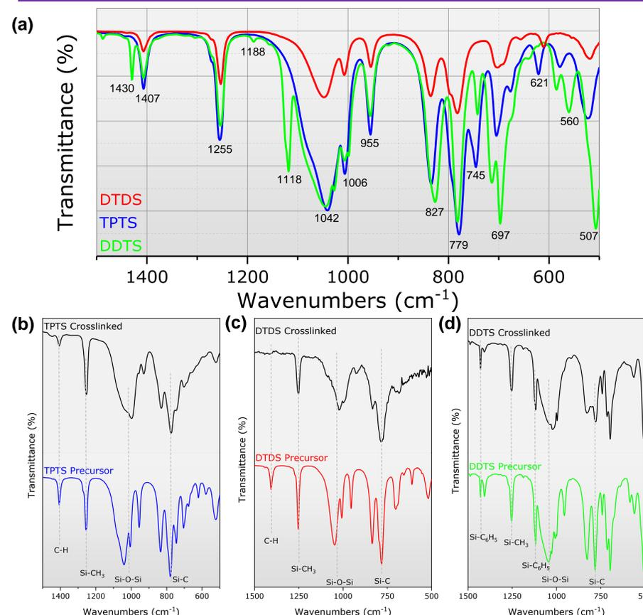
Fig 3: FTIR spectra of the precursor and crosslinked samples. Major peaks of crosslinked samples are labeled within the plot. (a) Comparison of chemical bonding between precursors (b) chemical bonding of TPTS (c) chemical bonding of DTDS (d) chemical bonding of DDTs.
