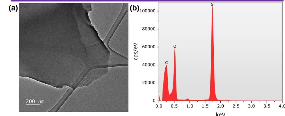
Fig 5: (a) TEM imaging of pyrolyzed TPTS particle (b) corresponding EDX spectra. Shows presence of elements Si, O, and C, as per expectation.
