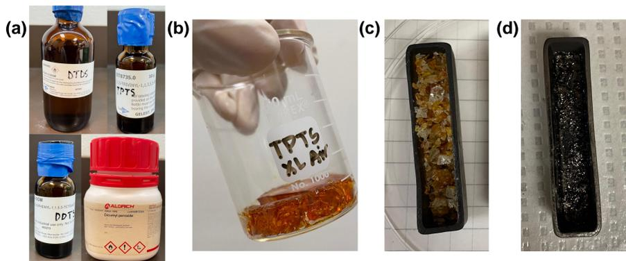
Fig 2: (a) DDTs, TPTS, DTDS precursors and DCP (b) crosslinked TPTS (c) TPTS after crosslinking (d) TPTS after pyrolyzing.
