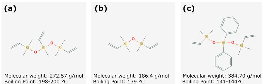
Fig 1: Molecular structure of precursors (a) TPTS (b) DTDS (c) DDTs.
