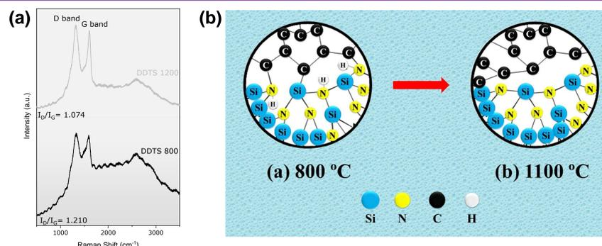
Fig 4: (a) Raman spectra of DDTs (b) independence of carbon phase<sup>4</sup>. Unclear peaks in 800°C indicates little formation of graphite, and more peaks under the ones shown. Clear peaks in 1200 °C indicate greater graphite formation. Decreasing peak ratio indicates more ordered carbon at higher temperatures.
