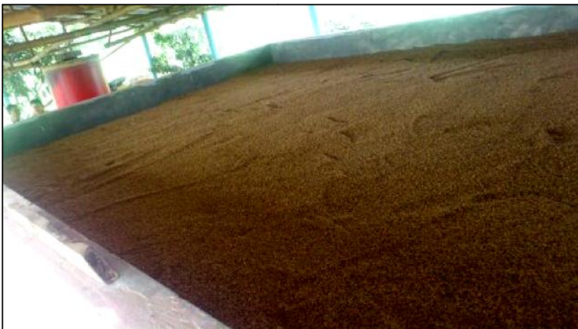
Photo 3: Parboiled paddy in bin being mechanically dried
