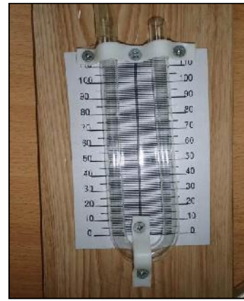
Figure 6: U-shape pressure meter
