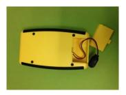
2. Attach the probe (this contains the sensor) to the meter by carefully pushing the handset plug into the plug adapter (located at the top of the meter) until a click is heard.
