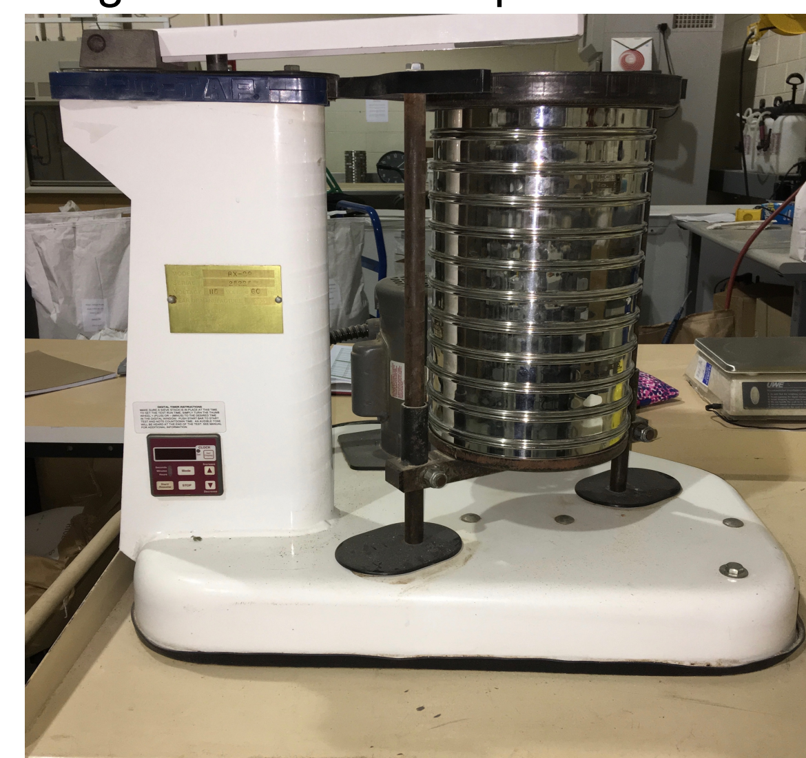
Figure 1. Rotational Tapping Particle Size Analysis machine (Ro-Tap II RX-94).
