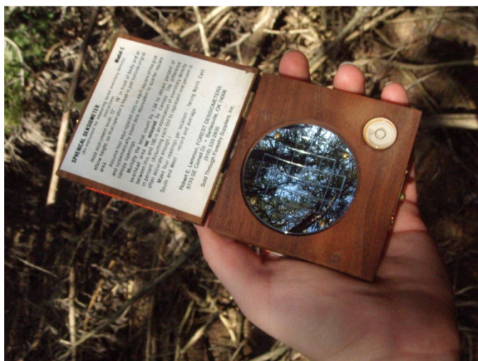
Figure 9. The densitometer measures percent canopy cover.
