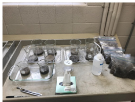
Image 1: Samples settling before decanting, a crucial step before being tested for particle size in the Mastersizer 3000.
