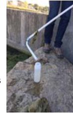
Image 2: The testing apparatus used to pull water samples.
