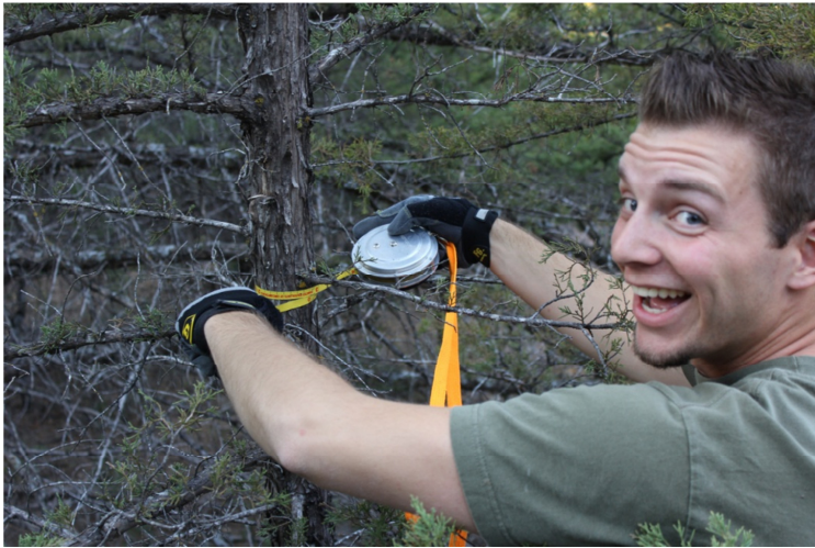
Figure 9: Demonstrating the use of a forester's measuring tape to determine the DBH of a tree.
