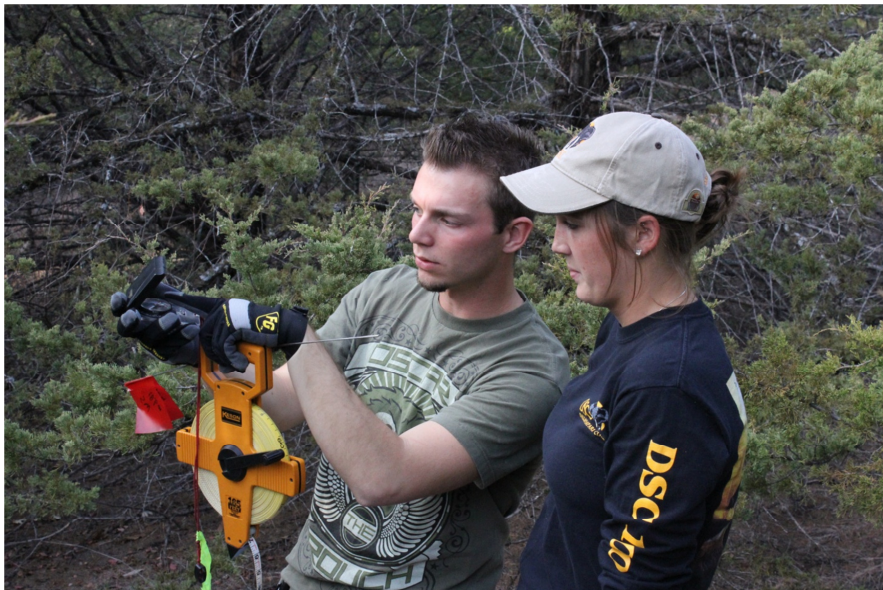
Figure 5: Field group members begin to lay out the study site using a compass, flags, and a measuring tape.
