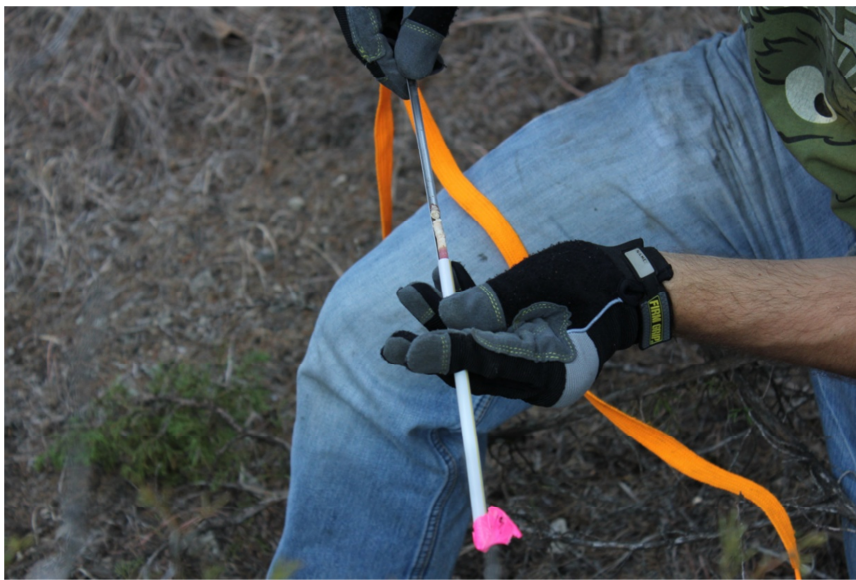
Figure 7: Showing the placement of the tree increment bore into a plastic straw for transportation to the lab.
