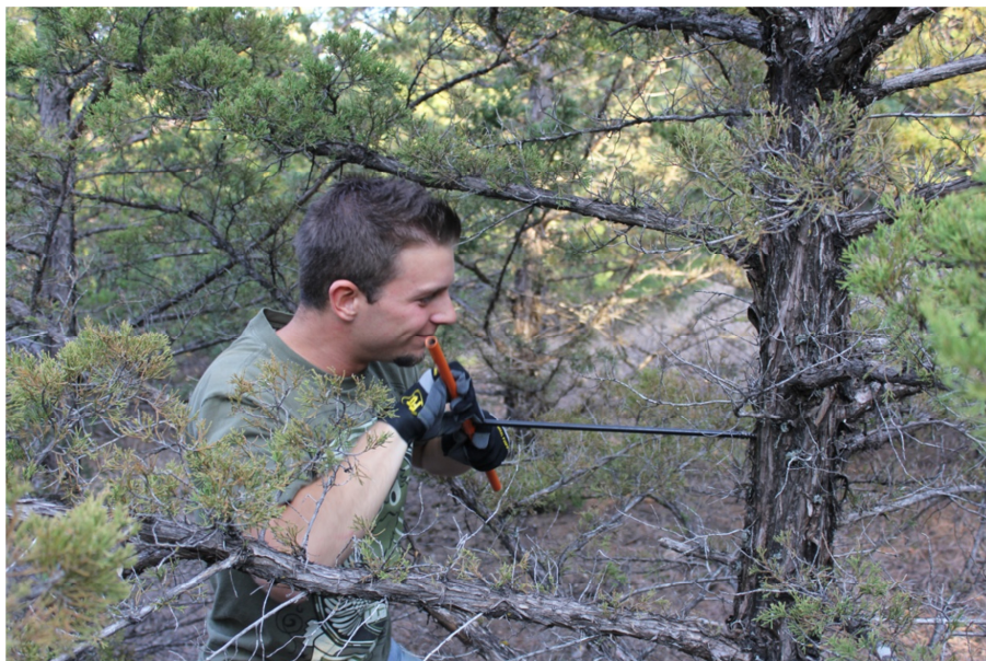
Figure 6: A field member using an incremental borer to remove the tree core samples, used later to count tree rings and estimate tree age.
