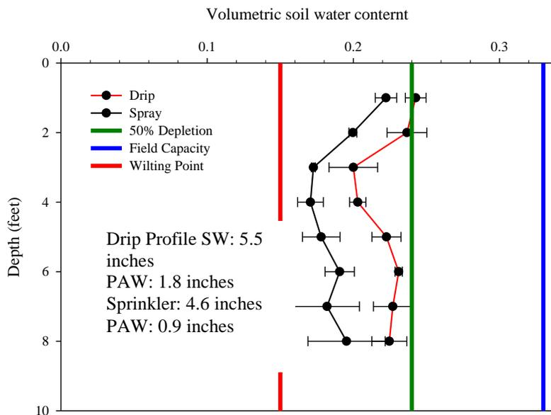
Figure 5. End of season soil water under Mobile Drip Irrigation (Drip) and Low Elevation Spray Application (Spray) for at high irrigation capacity of 4.6 gpm/ac during the 2015 growing season at the Kansas State University Southwest Research-Extension Center, near Garden City, Kansas (Kisekka et al. 2017).
