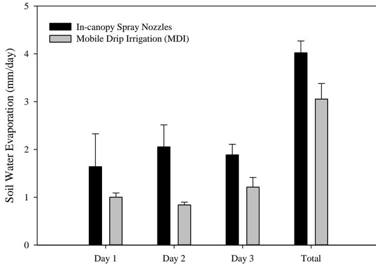
Figure 1. Comparing soil water evaporation under MDI and spray nozzles for three days during the 2015 corn growing season at the Kansas State University Southwest Research-Extension Center, near Garden City, Kansas.
