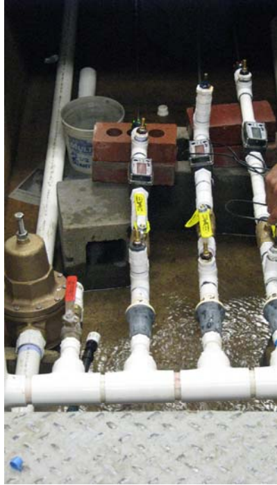
Figure 1. Picture of Pressure Regulator Test Stand, including manifold, pressure regulator, pressure shunt, water meter, pressure shunt and flow nozzle.
