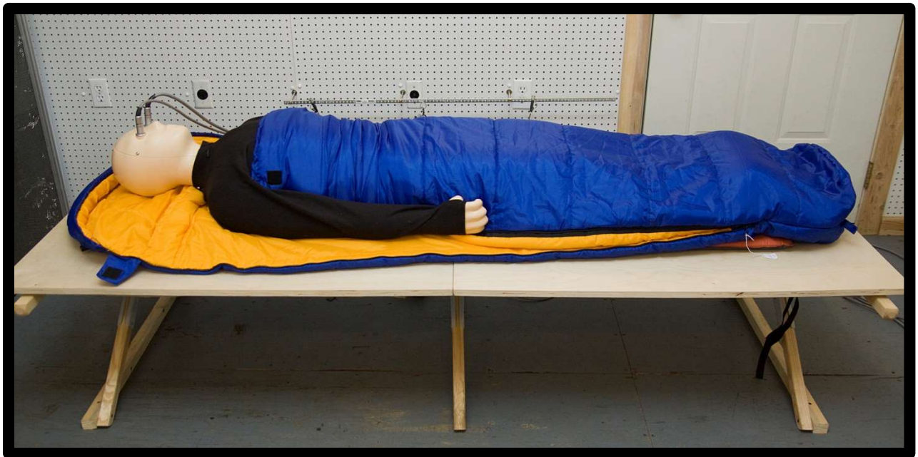
Optional ISO 23537 maximum comfort temperature test (posture #2). Note: This requires a second manikin test.
