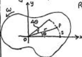
Rigid Object rotating about fixed axis  $O$  in  $z$ -direction
