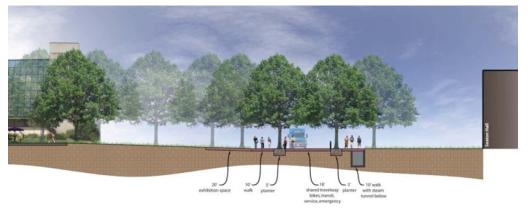
KSU 17th Street Multi-Modal Corridor Master Plan Section C Cross-Section - Transit/Bikeway Separated from Pedestrian Path
