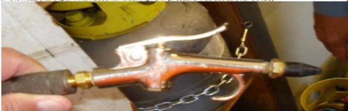
Condition: Compressed air shall not be used for deaning purposes except where reduced to less than 30 PSI and then only with effective chip guarding and personal protective equipment.
