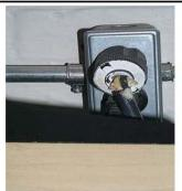
Figure 2 Wire Cover pulled from plug
