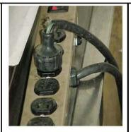
Figure 3 Plug pulled from casing & insulation
