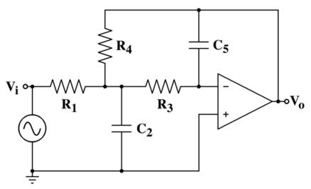
Sallen-Key Topology (non-inverting) (*some problems*) (<u>very</u> common) MFB Topology (inverting) (better imho) (less common)
