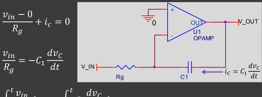
$$\int_0^t \frac{v_{in}}{R_g} dt = -\int_0^t C_1 \frac{dv_C}{dt} dt$$
