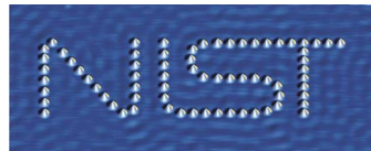
STM image of a 40-nm logo of NIST made with cobalt atoms, Science, 2004
