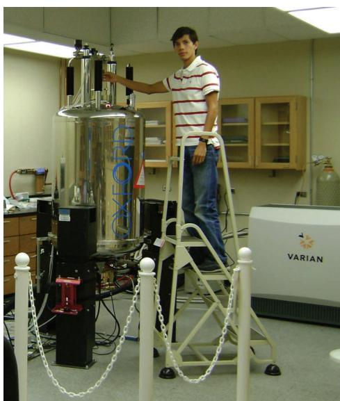
Facility Manager Alvaro Herrera testing the newly installed triple resonance cryogenic probe.
