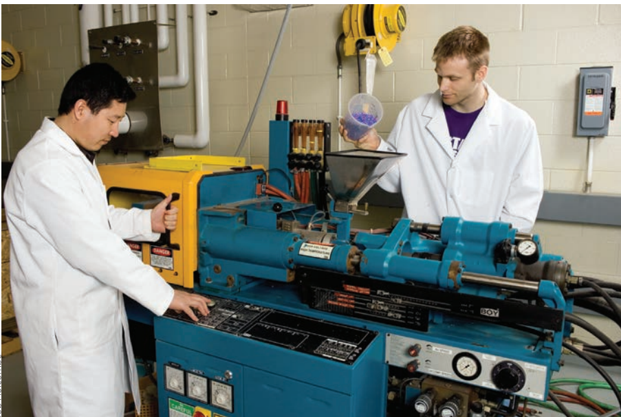
Staff at the BIVAP building use the Injection molder to produce plastics from renewable ag feedstock.
