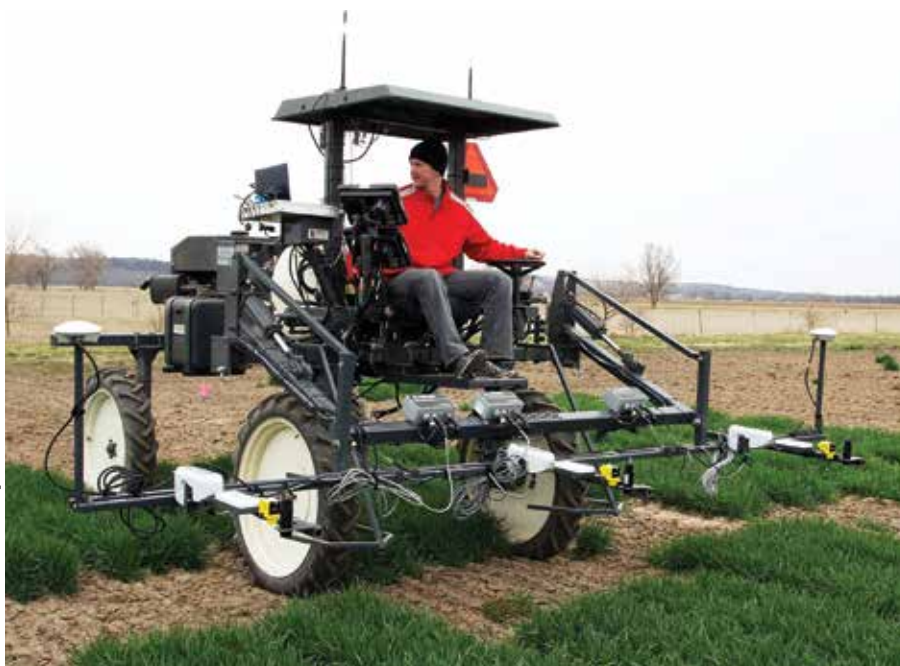
This small roving GPS-guided phenotyper, developed by a K-State research team, is equipped with cameras and sensors to gather and analyze plant data quickly as it moves through the field.
