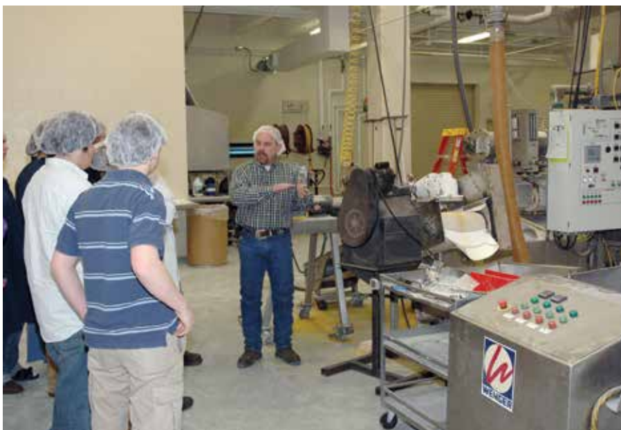
Eric Maichel, Bioprocessing and Industrial Value-Added Program operations manager, explains the grain extrusion process, which forces product through a dye to create a specific shape.
