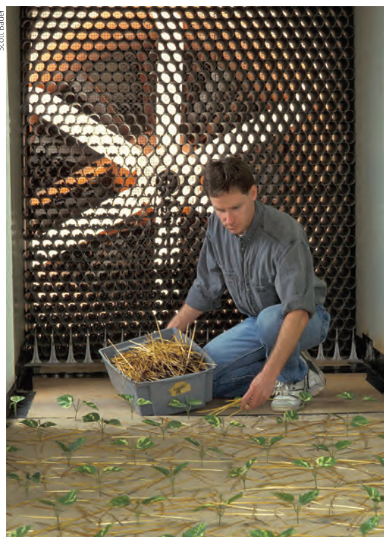
In a wind tunnel, technician Brent Schroeder prepares to measure how live plants and straw residue slow windblown soil erosion.
