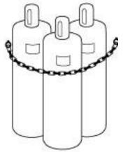
Figure 1 - example of proper three points of contact while storing gas cylinders
