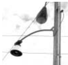
Figure 1. Omnidirectional Video Camera Mounted to Street Light Pole
