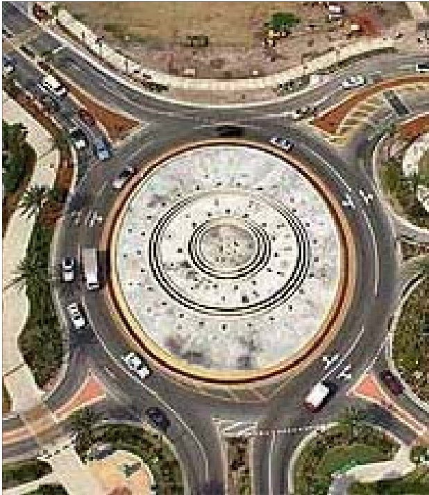
Figure 7. Clearwater Beach Roundabout After Striping and Curb Changes (Photo courtesy Ken Sides)
