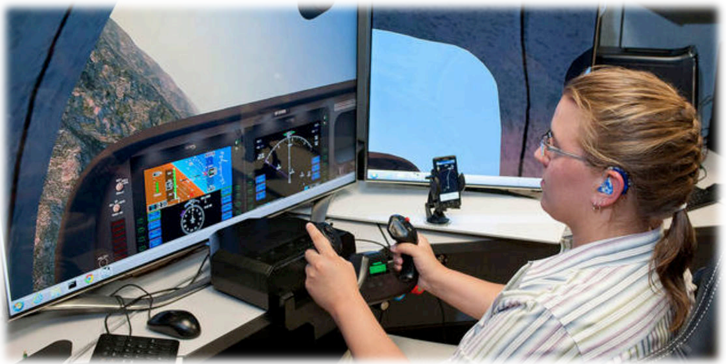
Computer science and engineering student Johanna Lucht pilots a plane simulator to test the collision avoidance on the Android phone app during her internship with NASA this past summer.
