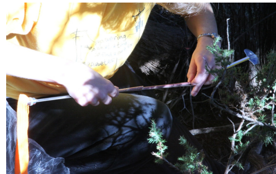
Figure 8. Tree core extraction using the Suunto tree borer.
