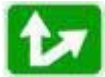
Figure 11: Sign indicating bicyclists may proceed right onto the multi-use path or straight to continue on road (Manual of Traffic Signs 2006).
