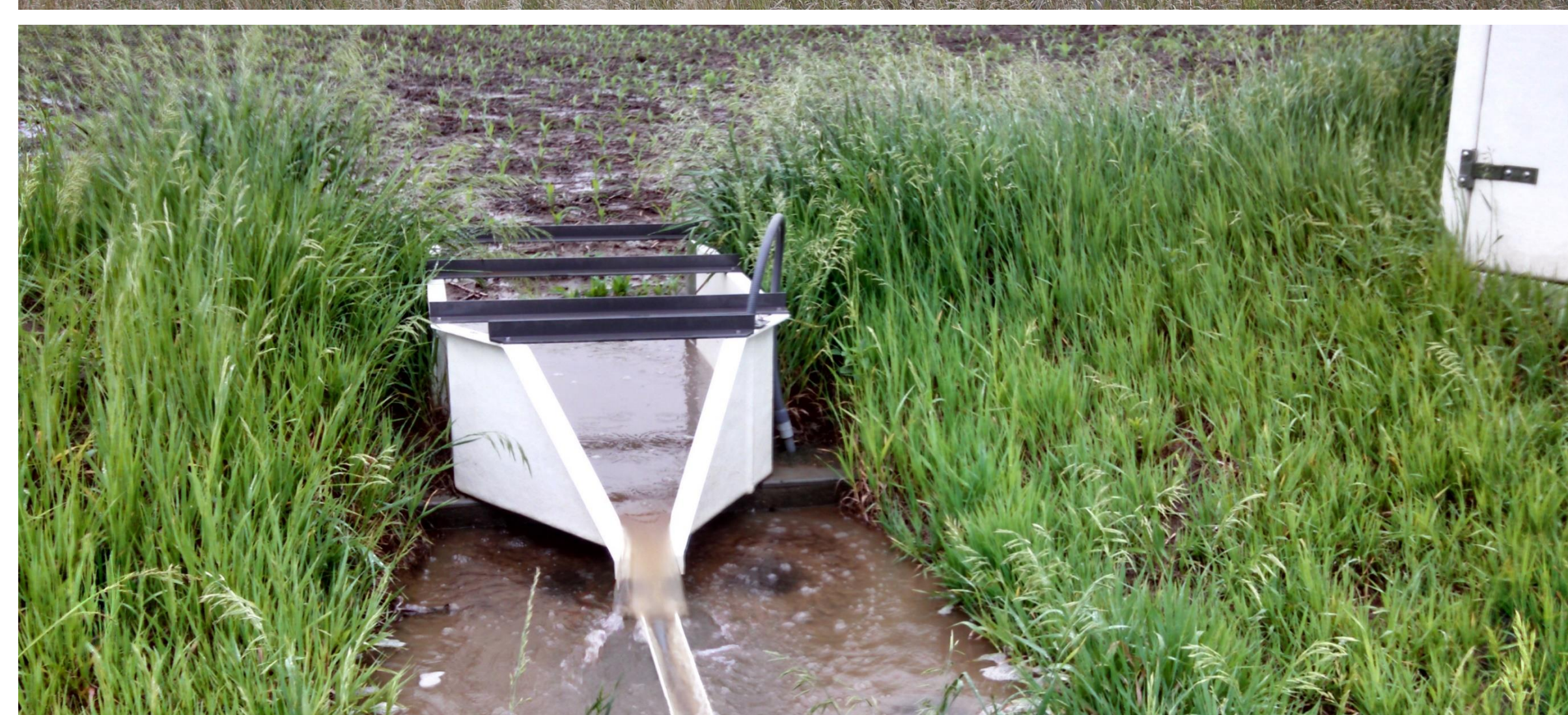
Figure 2. H-flumes and equipment for monitoring flow, collecting water samples, and monitoring precipitation at watershed outlets.
