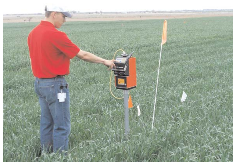
ARS engineer Jordan Varble measures soil water content down to 2 m depth in wheat with a neutron moisture meter.
