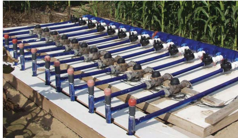
The irrigation control center for deficit irrigation trials at the ARS Limited Irrigation Research Farm near Greeley, Colorado. Irrigations are controlled through a data logger and measured with flowmeters.
