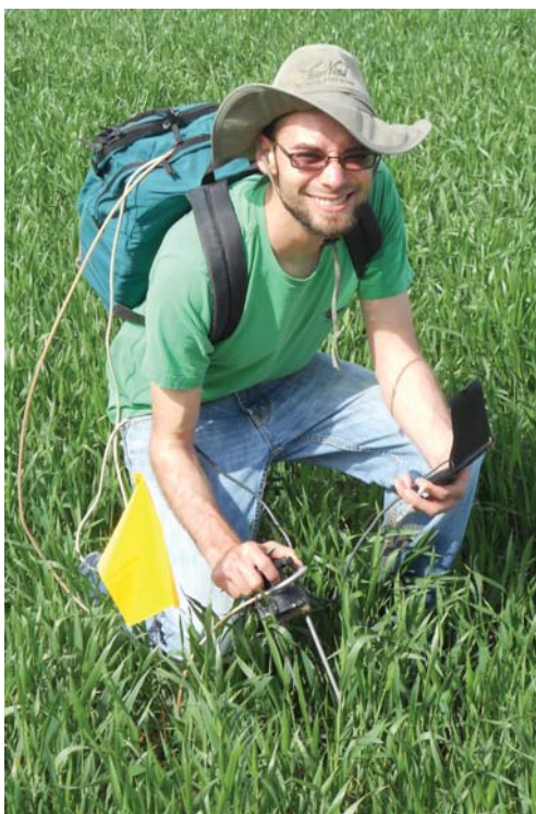
ARS engineer Garrett Banks measures soil water content in wheat with a portable TDR device.
