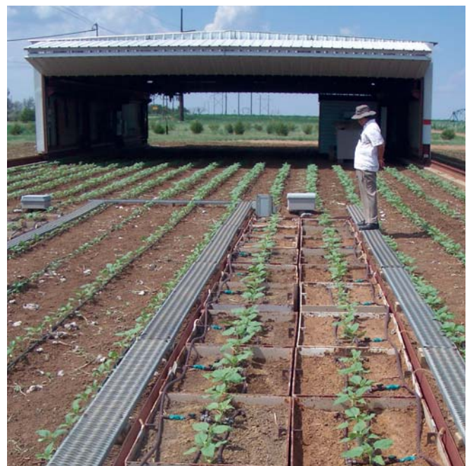
Sunflowers grow in mini-lysimeters at the ARS facility at Bushland, Texas. Several deficit irrigation treatments can be tested in a variety of soils in this lysimeter complex.
