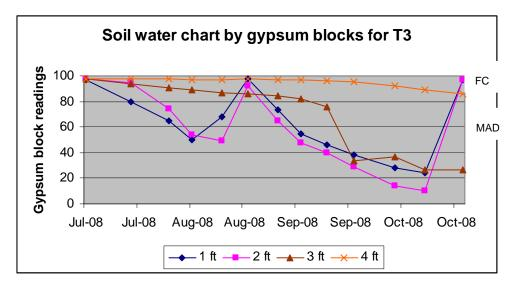
Fig. 6 shows soil water chart from readings obtained by gypsum blocks.
