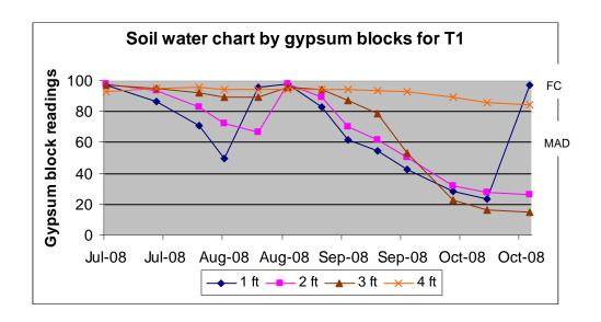
Fig. 5 shows soil water chart according to readings obtained by gypsum blocks.
