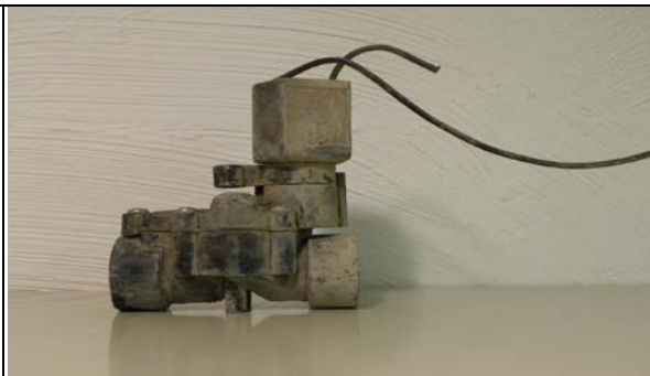
Figure 12. A broken solenoid wire on a zone valve might go unobserved if producers do not monitor their system flowrate and pressure.
