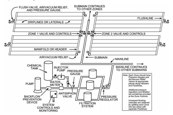
Figure 3. Schematic of a complete SDI system. After Lamm and Camp (2007).
