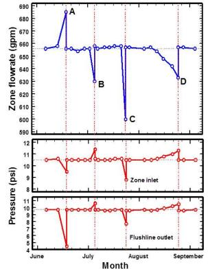
Figure 6. Hypothetical example of how pressure and flowrate measurement records could be used to discover and remediate operational problems. After Lamm and Camp (2007).
