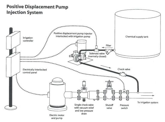
Figure 5. Layout of a chemical injection system with safety interlocks and backflow prevention devices (Courtesy of L.J. Schwankl, Univ. of California-Davis).
