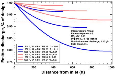
Figure 4. Calculated emitter discharge, emission uniformity (EU), and emitter discharge variation (q<sub>var</sub>) as affected by dripline length and emitter spacing (ES). Results for hypothetical dripline calculated with software from Roberts Irrigation Products (2003).
