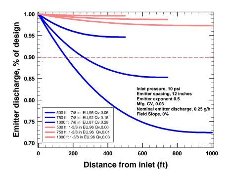
Figure 2. Calculated emitter discharge, emission uniformity (EU), and emitter discharge variation (q<sub>var</sub>) as affected by dripline length and inside diameter. Results for hypothetical dripline calculated with software from Roberts Irrigation Products (2003).
