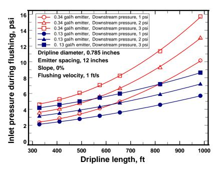
Figure 7. Required inlet pressure to maintain a 1 ft/s dripline flushing velocity, as affected by the nominal emitter discharge rate, dripline length, and downstream pressure. Results for hypothetical dripline calculated with software from Toro Ag Irrigation (2002).
