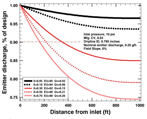
Figure 6. Calculated emitter discharge, emission uniformity (EU), and emitter discharge variation ( $q_{var}$ ) as affected by the emitter exponent (x). An emitter with an exponent of zero is said to be fully pressure compensating (PC). Results for hypothetical dripline calculated with software from Roberts Irrigation Products (2003).
