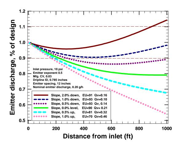
Figure 5. Calculated emitter discharge, emission uniformity (EU), and emitter discharge variation  $(q_{\text{var}})$  as affected by topography. Results for hypothetical dripline calculated with software from Roberts Irrigation Products (2003).
