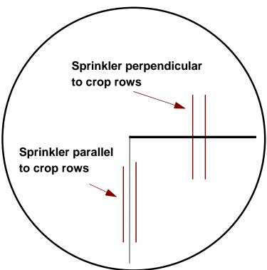
Figure 8. Two problematic orientations for in-canopy sprinklers when crops are not planted in circular rows.
