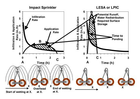
Figure. 3. Illustration of runoff or surface water redistribution potential for impact and LESA sprinkler application packages for an example soil. After Howell (2006).
