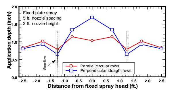
Figure 9. Differences in application amounts and application patterns as affected by corn row orientation with respect to the center pivot sprinkler lateral travel direction. Dotted lines indicate location of corn rows and stemflow measurements. Data are from a fully developed corn canopy, July 23-24, 1998, KSU Northwest Research-Extension Center, Colby, KS. Data are mirrored about the centerline of the nozzle.
