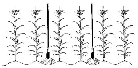
Figure 4. LEPA concept of equal opportunity of plants to applied water. LEPA heads are centered between adjacent pairs of corn rows. Using a 5–ft nozzle spacing with 30-inch spaced crop rows planted circularly results in plants being approximately 15 inches from the nearest sprinkler. After Lamm (1998).
