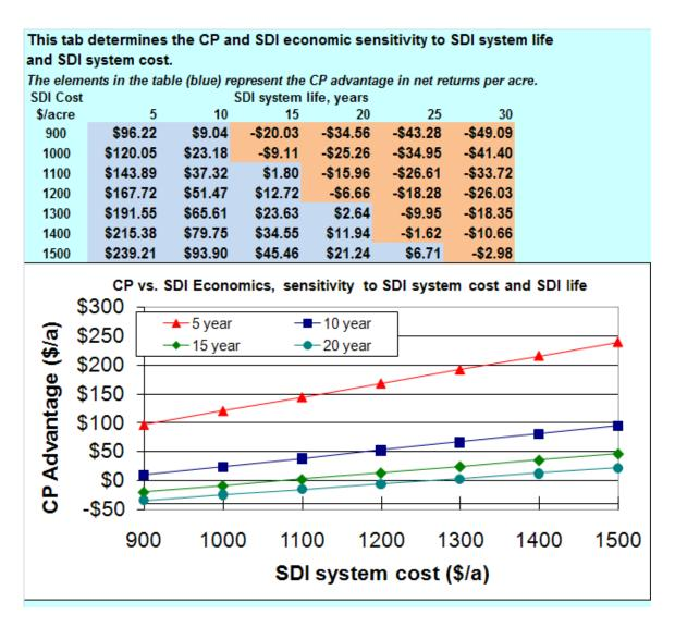
Figure 5. The SDI cost and life worksheet (tab) sensitivity analysis. Note this is one of three worksheets (tabs) providing tabular and graphical sensitivity analyses. These worksheets automatically update to reflect changing assumptions on the Main worksheet (tab).
