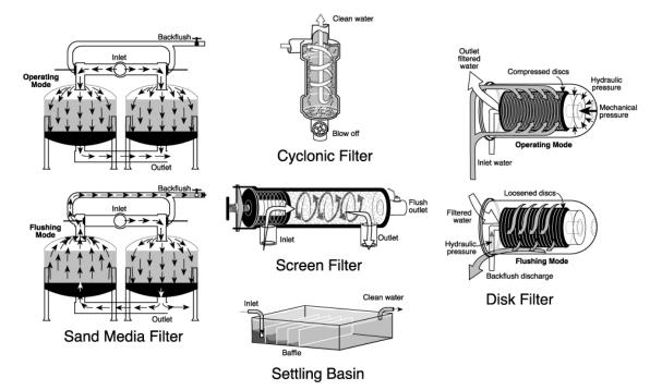
Figure 4. Schematic description of various filtration systems and components. (Courtesy of Kansas State University).
