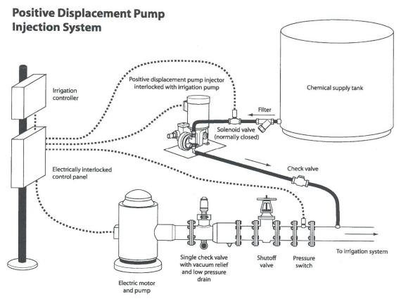
Figure 5. Layout of an Injection System with Safety Interlocks and Backflow Prevention Devices (Courtesy of L.J. Schwankl, Univ. of California-Davis)
