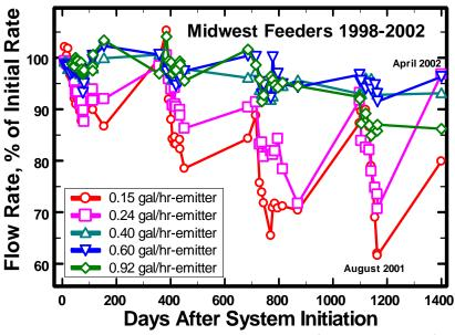
Figure 15. Decrease in emitter discharge during four seasons of operation of an SDI system with biological effluent at Midwest Feeders, Ingalls, Kansas, 1998 to 2002.
