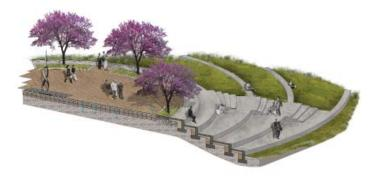
Mid-Campus Plaza The plaza utilizes permeable paving and structural cells, which allow stomwater to infiltrate directly through the surface and into soil below.
