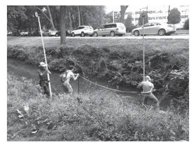
To create a longitudinal profile of the creek, we took to the field for data collection. Landscape architecture and engineering students measured stream bed depth and surface water elevation at key locations. Professor Keane illustrated surveying methods, then students took the reins to complete surveying of the entire stream.
