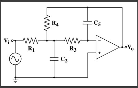
Sallen-Key Topology (non-inverting) (some problems) (very common) MFB Topology (inverting) (better imho) (less common)
