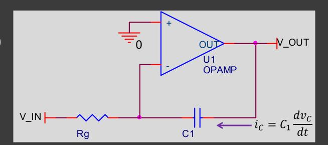
$$\int_0^t \frac{v_{in}}{R_g} dt = -\int_0^t C_1 \frac{dv_C}{dt} dt$$
