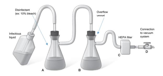
Figure 1 Vacuum System Protection (adapted from the BMBL, 5th Ed, 2009, pg322).
