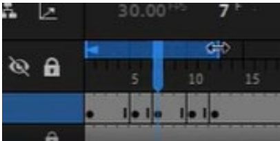
Figure 18. Loop Markers Define and Limit the Looping Sequence (See the Blue markers above the timeline.)
